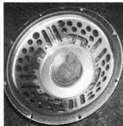
Preparing to remove the voice coil.
