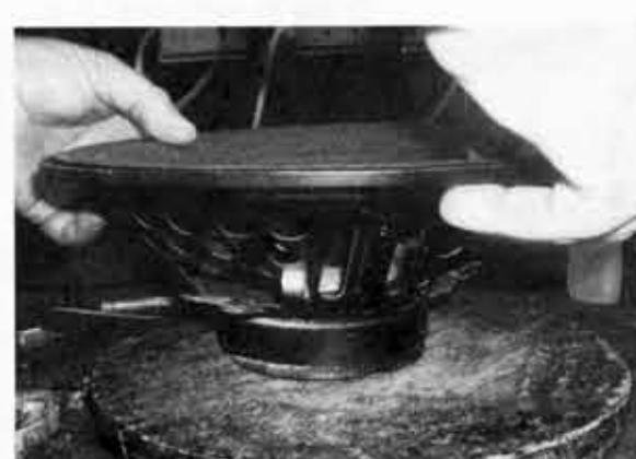
Placing the cone in the frame.
