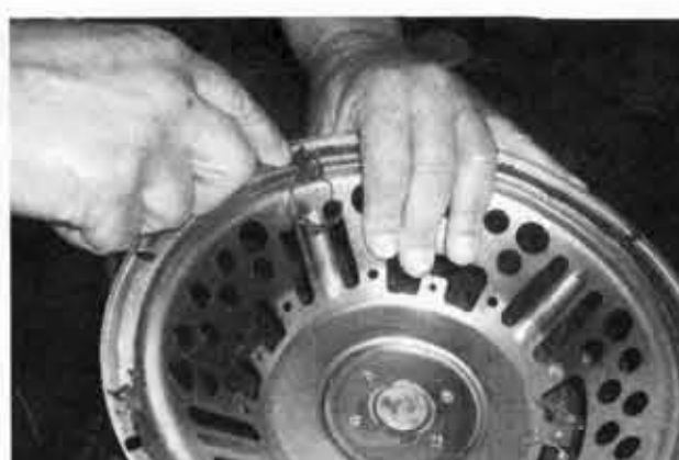
Scraping the frame.
